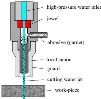
Fig. 1. Schematic drawing of the AWJ process.
