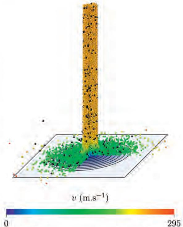
Fig. 4. Example of  $\frac{3}{4}$  of AWJ granular medium and its velocity field simulated just after impact, with 10 mm of canon/work-piece distance and 5 % of volumic ratio of abrasive particles. These last ones are drawn in black.
